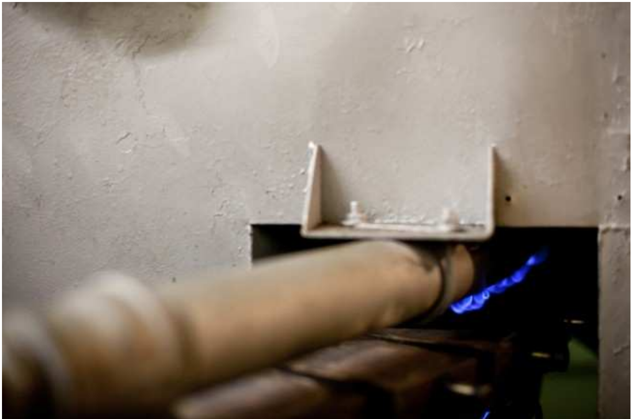
The batter is clamped shut inside a cooking surface similar to a Japanese kata and directed into a tunnel of gas flames.
