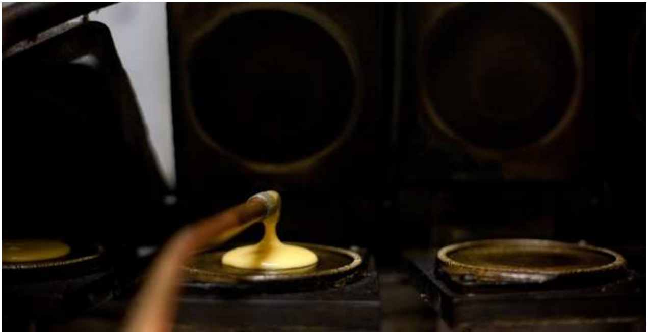
A spout adds just enough batter to the cooking surface.
