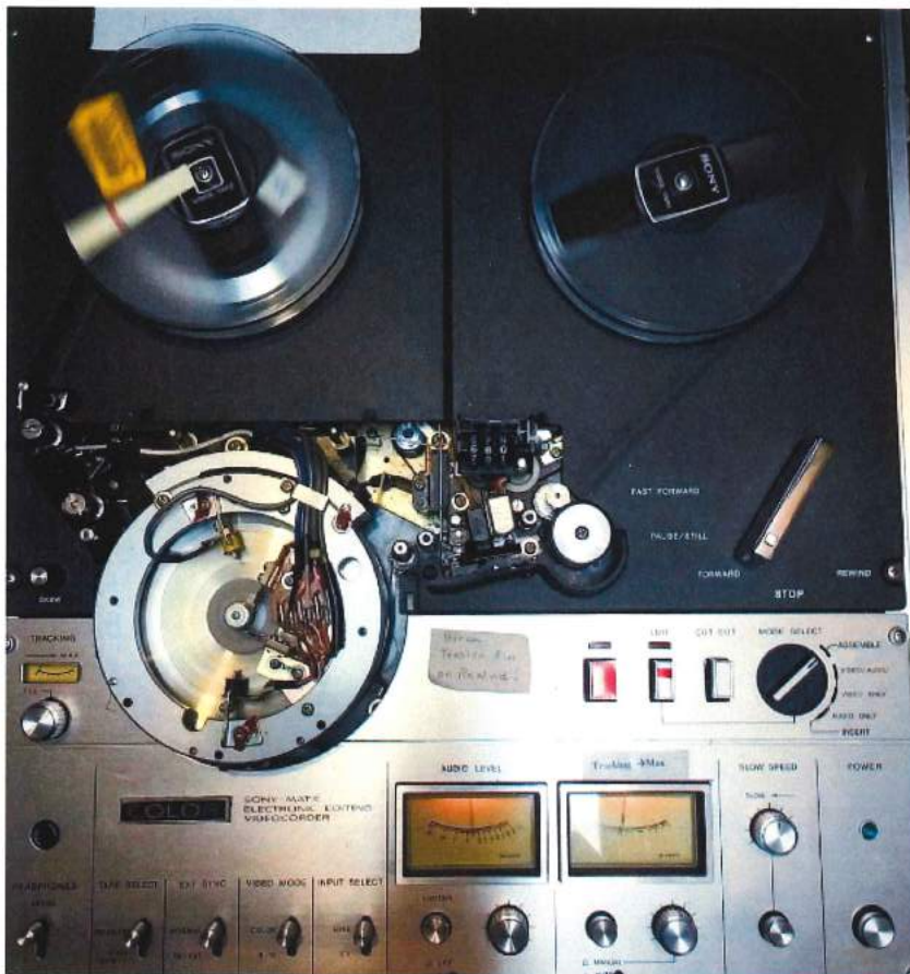
Below: A machine in BAVC's Preservation Suite, playing back a 1/2" open-reel video recording, originally recorded on Portapak
