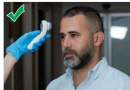
Figure 1: Correct Use – Forehead unobstructed, and NCIT perpendicular to forehead and used at distance identified in manufacturer's instructions.
