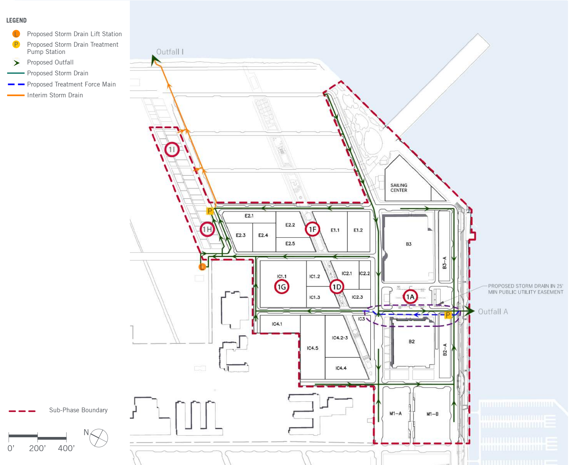
FIGURE 5.2 SUB-PHASE STORM DRAINS
