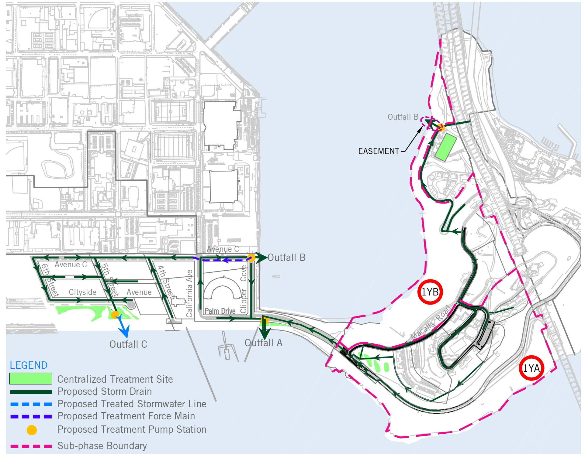
FIGURE 5.1 SUB-PHASE STORMWATER TREATMENT
