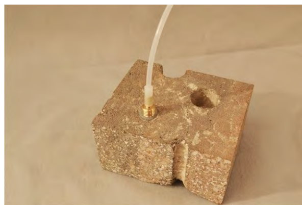
Figure 5. Vapor Pin™ sample connection.
