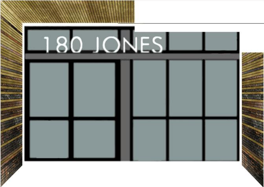
Tile layout design on the walls and ceiling of the main entryway using Ann Sacks "Elenco" series porcelain gold and nero tiles cut to 2" strips.
