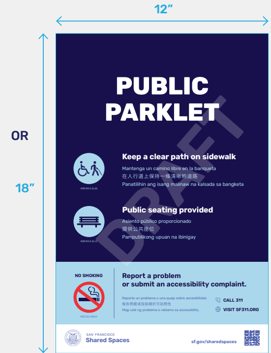
1/8" Anodized aluminum wrapped with laminated digital print. Applied white copy - reflective.
