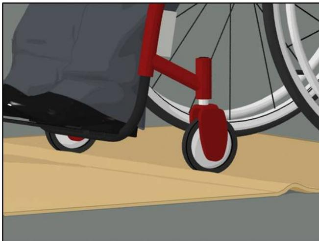
*Carpeting must be securely attached so that it does not shift or buckle against wheeled traffic. Cushions or pads, if used, also must be properly secured to resist movement. Rolling or buckling occurs when carpet is not properly secured and makes wheelchair maneuvering very difficult.*
