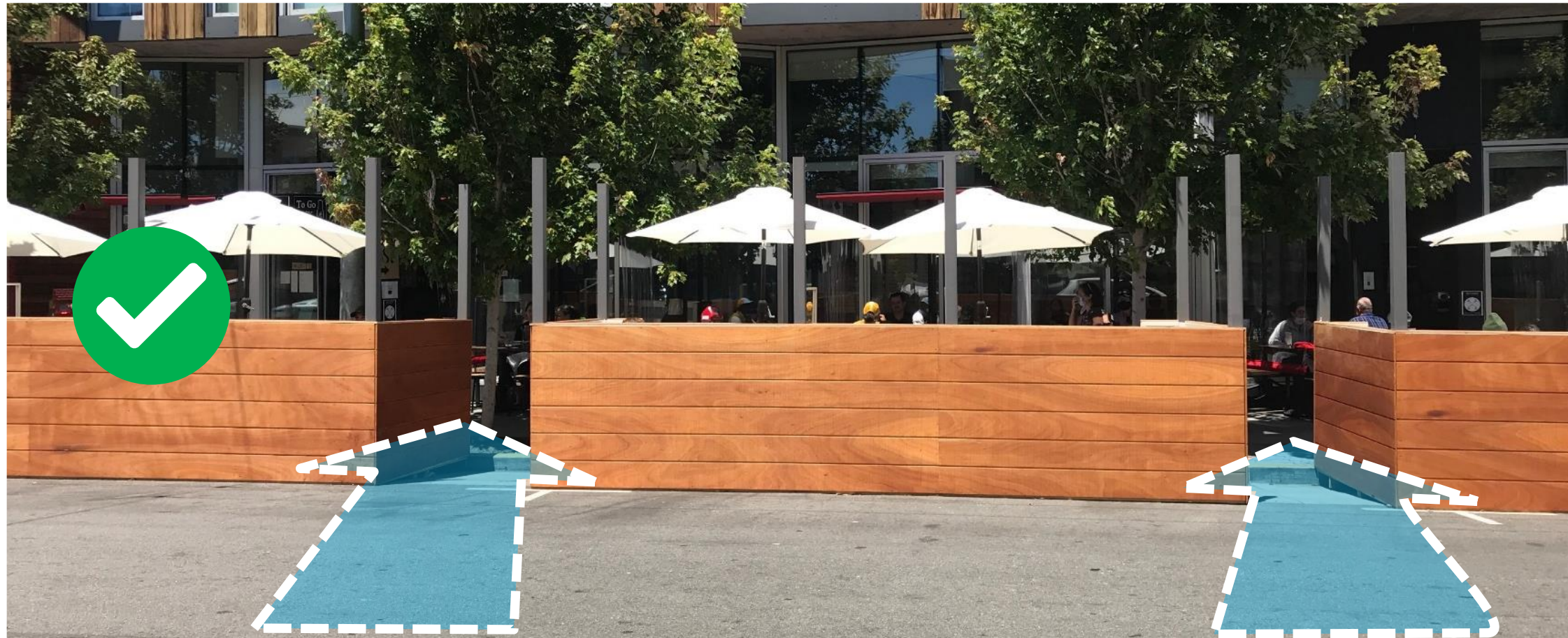
Gaps, open to the sky, for firefighter and paramedic access
