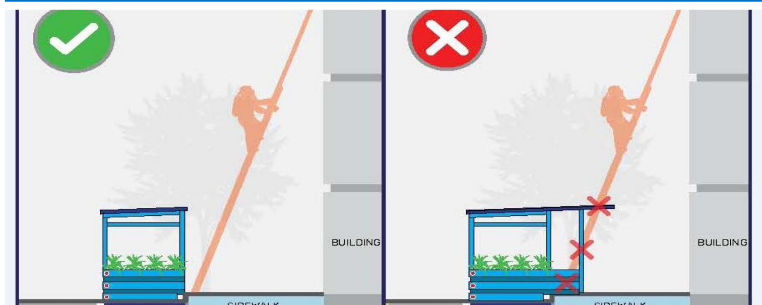
Clearance for Firefighting Ladders
