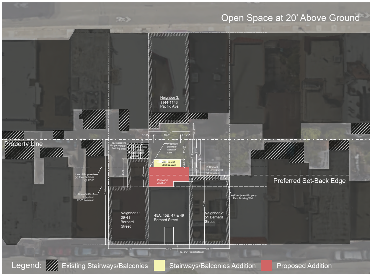
Figure Three: Site view of the existing open space, with the proposed addition (in red), and the proposed balconies and stairs (in yellow)
