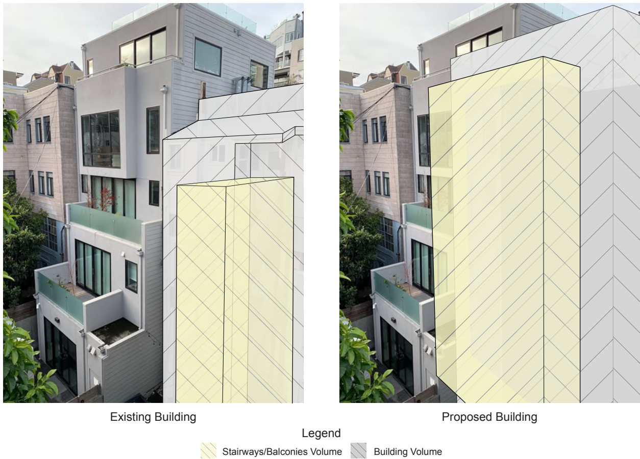
Figure Four: Renderings of existing rear elevation and the proposed elevation of 45-49 Bernard Street
