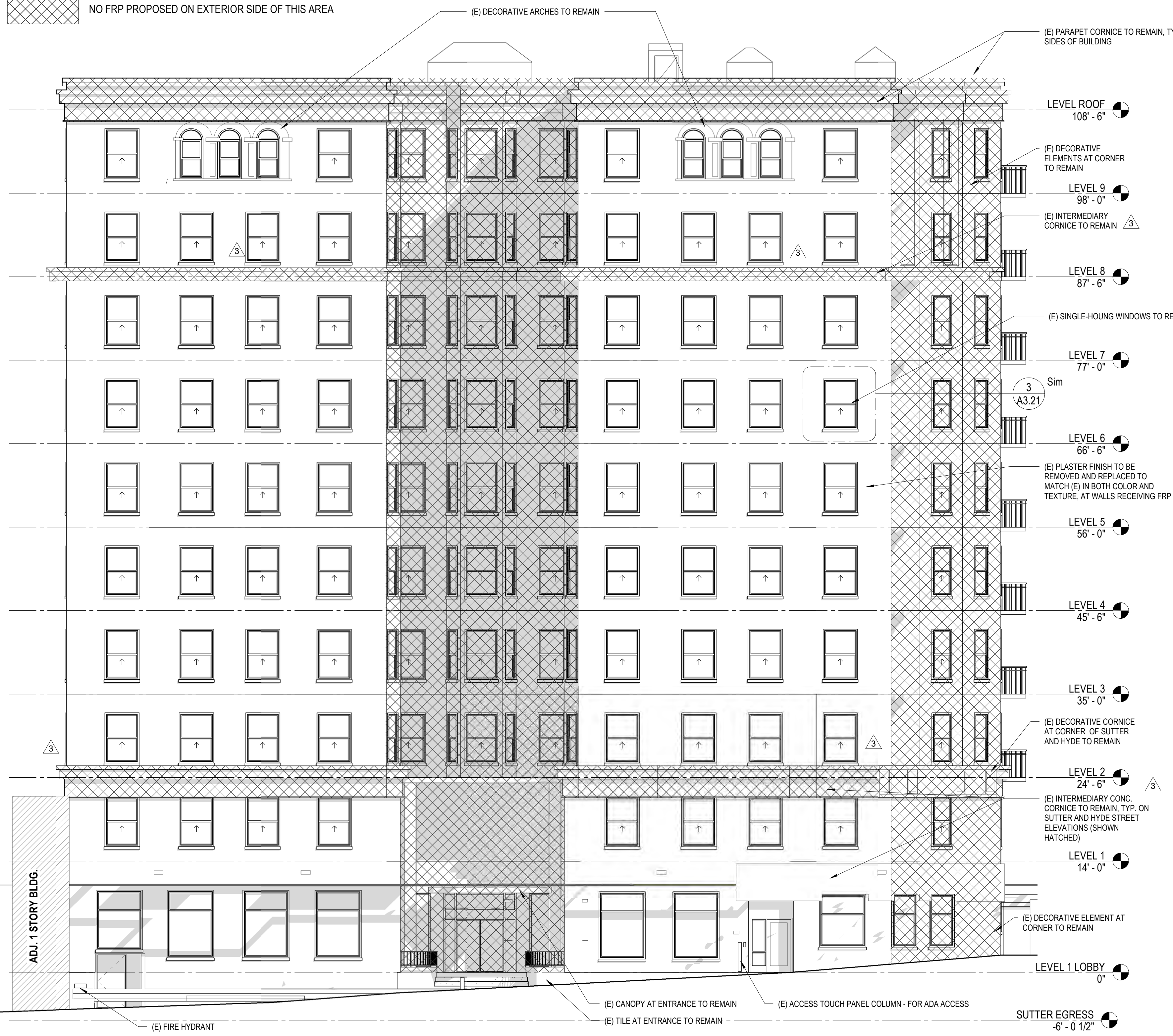
1 SOUTH (SUTTER ST) ELEVATION - NEW CONSTRUCTION 1/8" = 1'-0"
