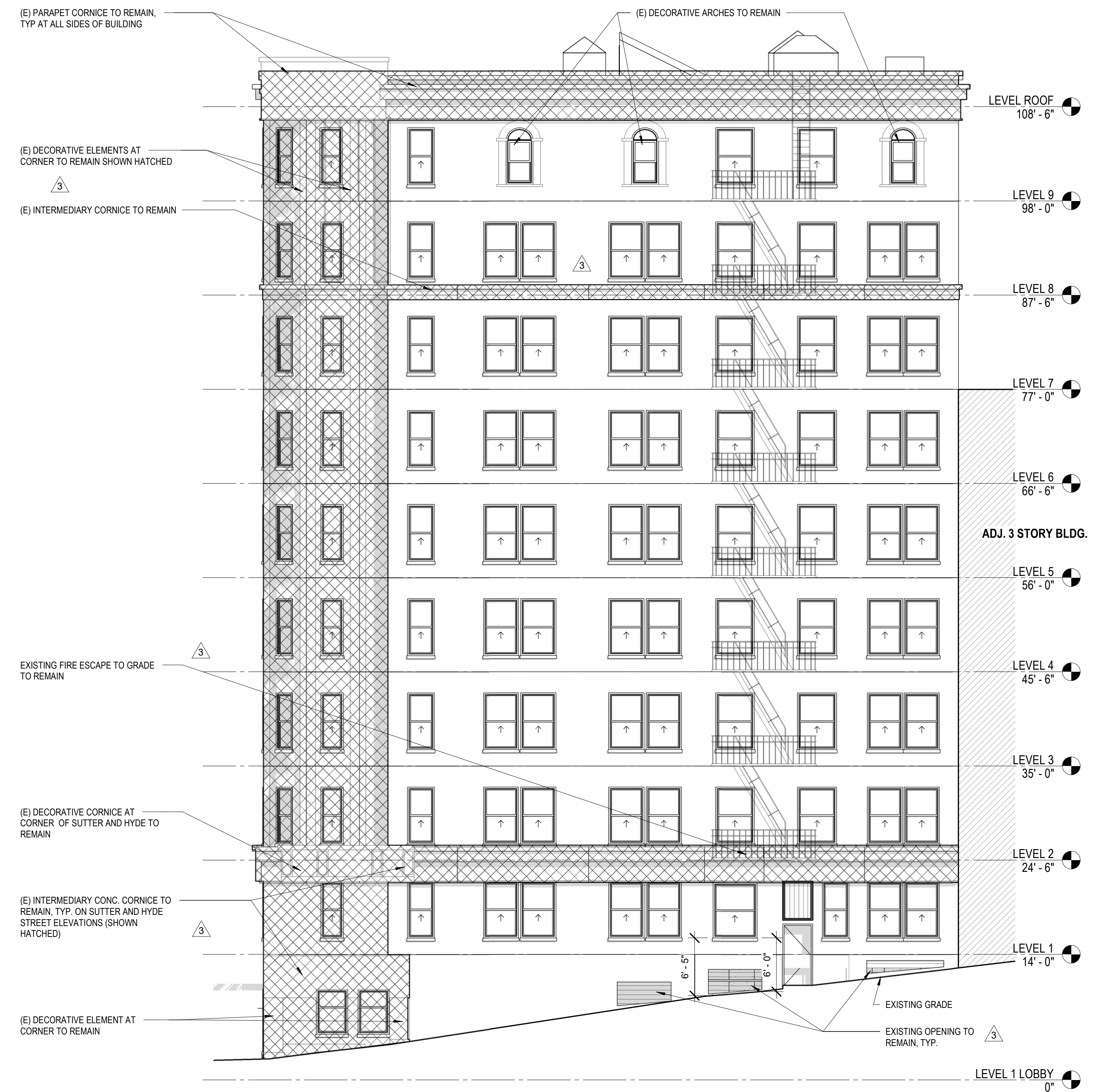
2 EAST (HYDE ST) ELEVATION - NEW CONSTRUCTION 1/8" = 1'-0"
