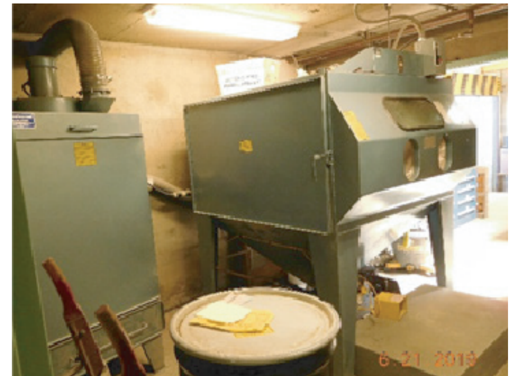
Old B-Blasters in most shops in a confined space with inadequate ventilation. No containment of debris.
