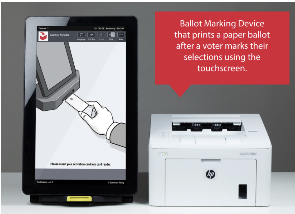
The Dominion ICX BMD consists of an off-the-shelf tablet and laser printer.
